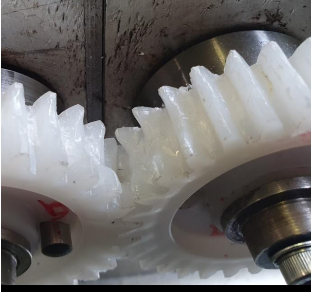
Fig 5.32 Melting of gear teeth at width centre.
