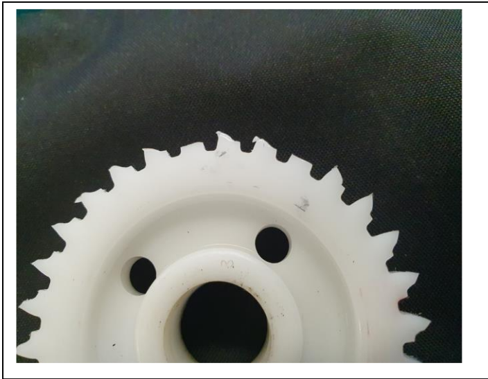
Fig 5.25 Detachment of teeth for 65°C gears at 3 Nm, 1000 rpm.
