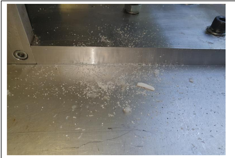
Fig 5.24 Debris at failure for 65°C mould temperature
