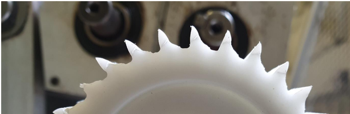
Fig 5.20 Cracked driving teeth still attached to gear at failure.
