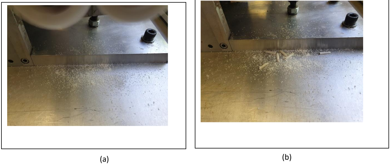
Fig 5.38 (a) 65°C gear debris at 0.8 \times 10^6 cycles. (b) Debris at failure.
