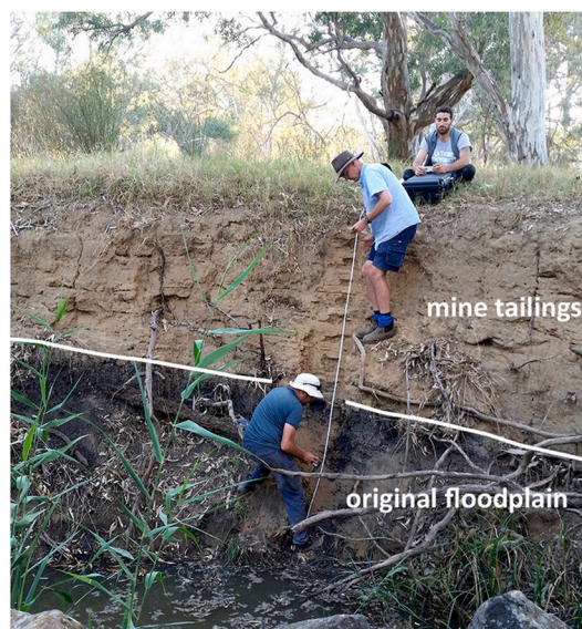
Fig. 4. Legacy sediment showing lighter brown mine tailings overlying darker pre-European floodplain deposits, River Loddon, Victoria, Australia.
