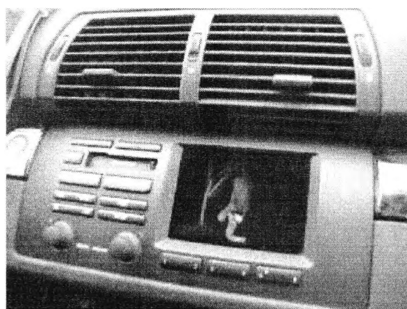
Figure 6.3: Displaying of processing results from embedded DSP via car on-board monitor.
