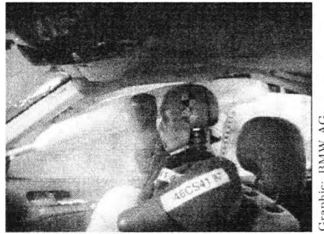
Figure 1.2: Crash with crash dummy. Demonstration of airbags for side impacts.
