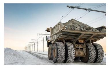
CAT Trolley Assist: diesel –electric overhead catenary mining trucks
