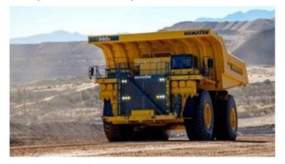
Komatsu: hydrogen fuel cell powered dump truck
