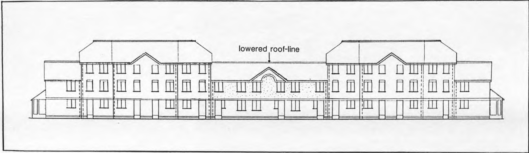
FIGURE 4.3 Front elevation of housing block "F", Surrey Waters, London, showing lowered roof-line of middle section (source: adapted from 1:200 block elevation drawing, Diamond Partnership architects, 1985)
