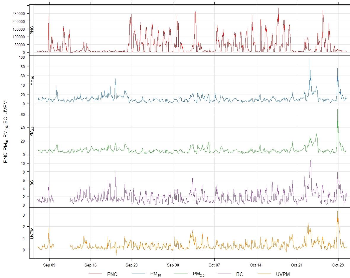
Fig S3 | Hourly timeseries data for LHR2, Sep-Oct 2019. PM 10 , PM 2.5 Black Carbon and UV Particulate Matter (UVPM) are all in units of μg/m 3 , Particle Number Concentrations in #/cm 3
