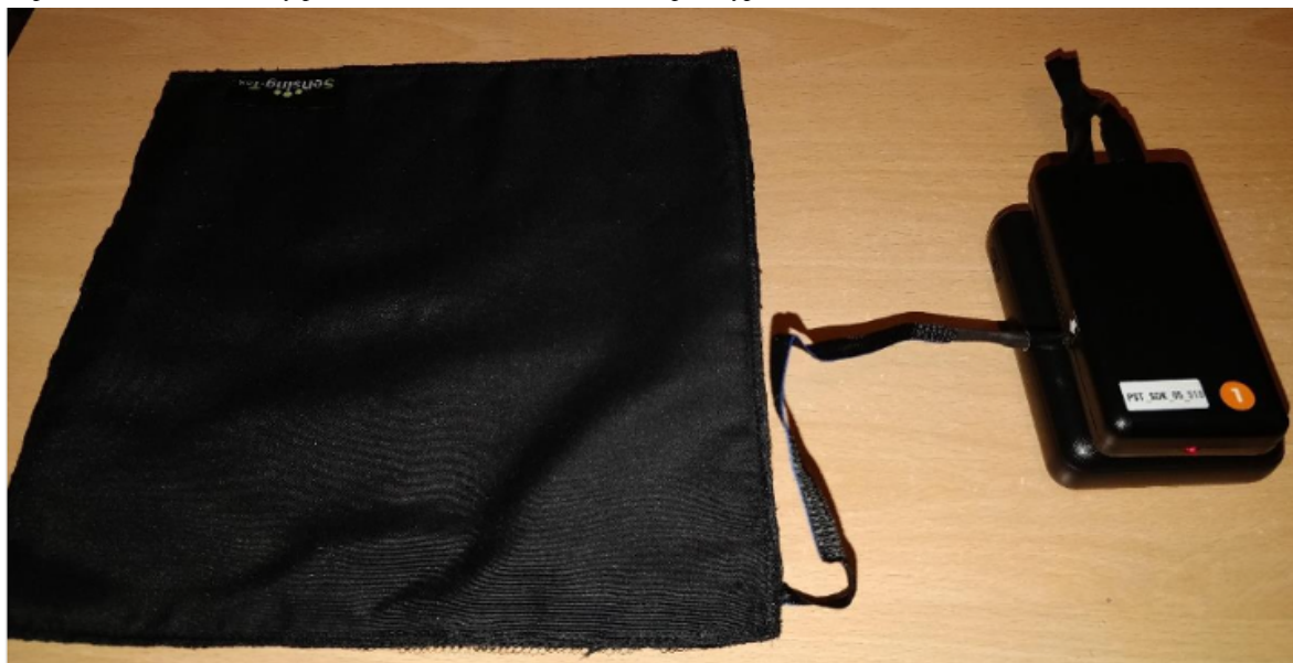
Figure 2. A pressure mat and a battery pack that were used as a basis of the prototypes.
