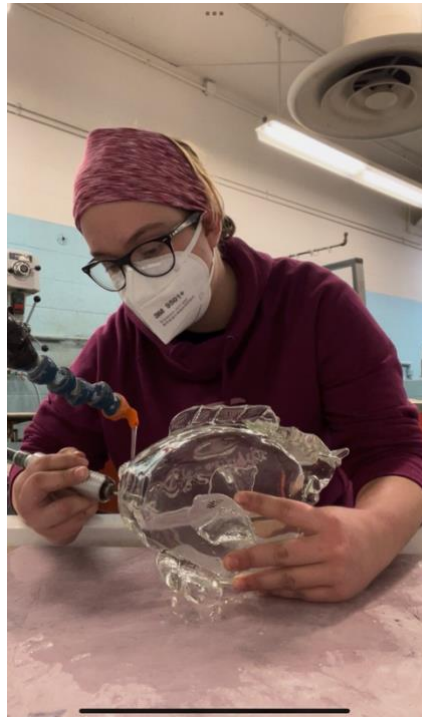
Figure 5.3: Practicing good safety in the cold shop. Loose articles tucked away, hair pulled up, glasses, and mask.
