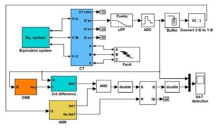
*Fig. 5.* MATLAB-Simulink based model for current transformer saturation detection with a use of proposed combined method
