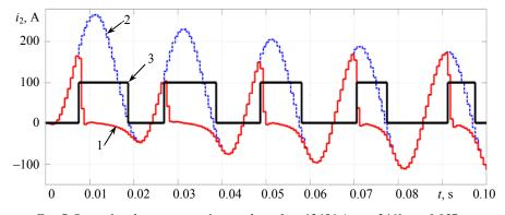
*Fig. 7.* Saturation detector operation results at  $I_{sc} = 12456$  A,  $\varphi = 346^\circ$ ,  $\tau = 0.057$  s: 1 – real current transformer secondary current; 2 – ideal current transformer secondary current; 3 – saturation detector output signal
