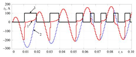
*Fig. 8.* Saturation detector operation results at  $I_{sc} = 15850$  A,  $\varphi = 133^{\circ}$ ,  $\tau = 0.033$  s: 1 – real current transformer secondary current; 2 – ideal current transformer secondary current; 3 – saturation detector output signal
