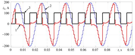
*Fig. 6.* Saturation detector operation results at  $I_{sc} = 16547$  A,  $\varphi = 90^{\circ}$ ,  $\tau = 0.065$  s: 1 – real current transformer secondary current; 2 – ideal current transformer secondary current; 3 – saturation detector output signal
