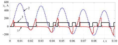
*Fig. 9.* Saturation detector operation results at  $I_{sc} = 44543$  A,  $\varphi = 16^{\circ}$ ,  $\tau = 0.072$  s: 1 – real current transformer secondary current; 2 – ideal current transformer secondary current; 3 – saturation detector output signal
