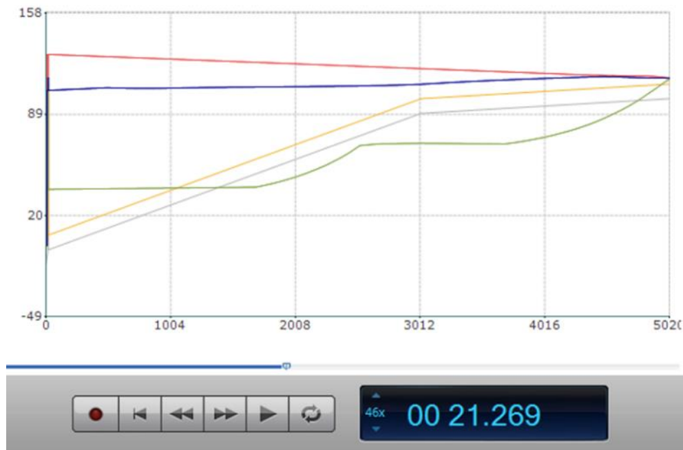
Figure 13. Result of no negative pressure, no cavitation after 21 s
