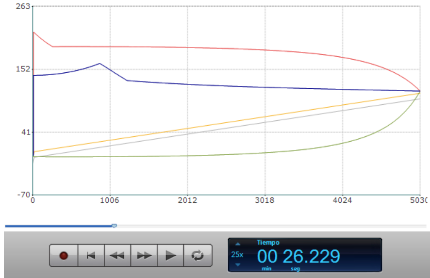
Figure 7. Negative pressure, cavitation and high pressure (220m) after 26 s
