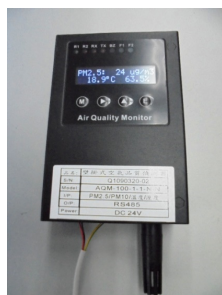
(a) Integrated temperature, humidity, and PM sensor
