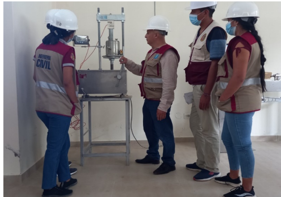
Fig. 1 Application of the overburden on the soil sample
