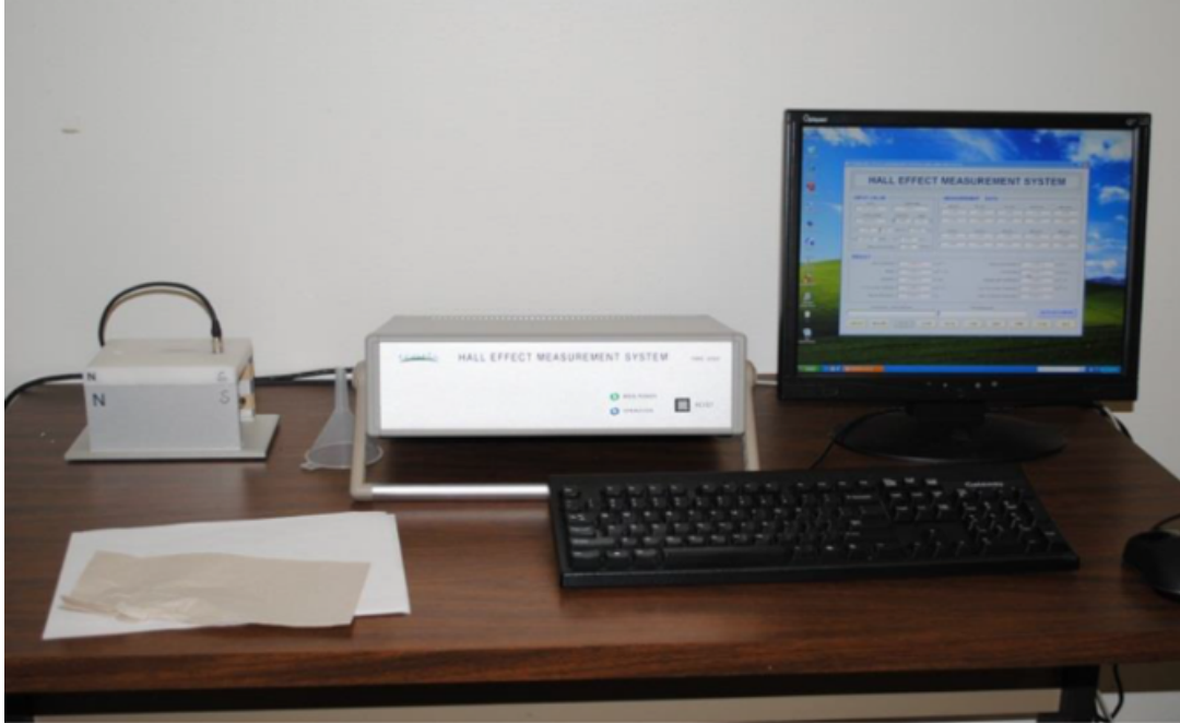
Figure 15: Hall effect measurement system in USD lab.
