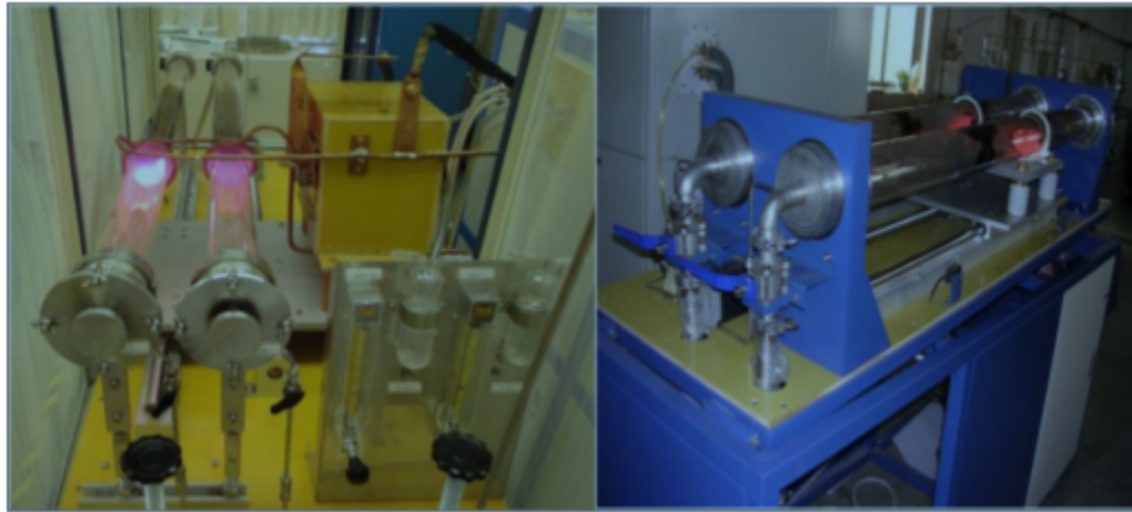
Figure 5: Zone refining set up in USD lab.
