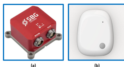
Figure 2. IMU devices used for validation: (a) SBG Ellipse-E; (b) MetaMotionR.
