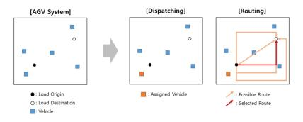
Figure 1. Dispatching and Routing Problems in AGV
