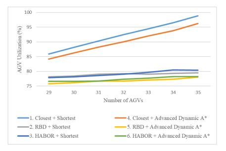
Figure 6. Utilization According to the Number of AGVs
