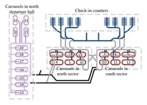
Figure 7. Layout of Baggage Unloading Carousels
