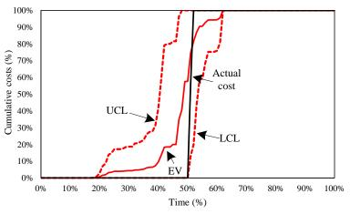
Figure 6. EV of the budget percentage and cost control limits for work item D03G35.
