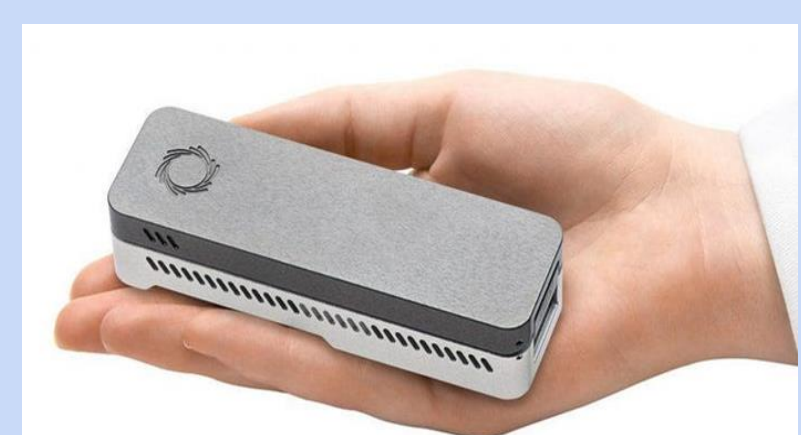
Fig 1. Portable Nanopore MinION device used to obtain DNA sequences (University of Oxford, 2015).
