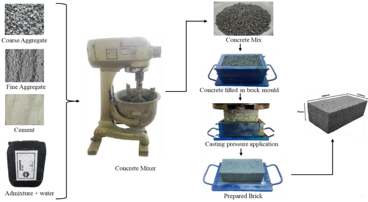
Fig-2: Manufacturing process of RAC Bricks
