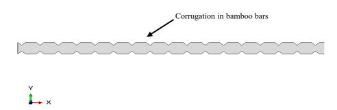
Fig -2: Corrugated Bamboo used for Modelling.
