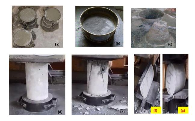
Fig-2: (a) Casting of concrete cylinders (b) Particle size of cement/fly ash (c) slump test (e) Compression testing (f) and (g) Split tensile testing
