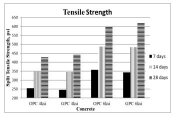
Fig -5: Tensile strength at 7, 14, 28 days
