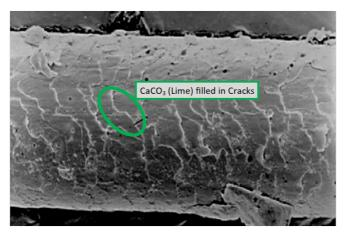
Fig -3: SEM Test of Healing
