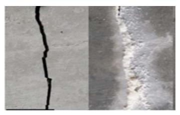
Fig -1: Healing of Crack [2]
