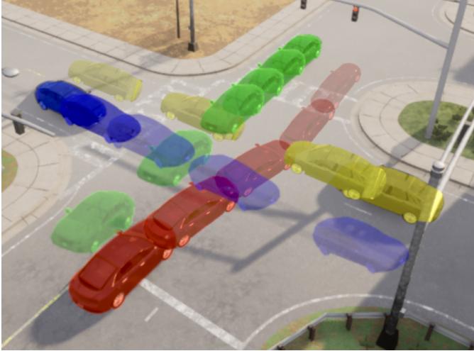
Fig. 8: Trajectories generated by STCS for Scenario N2 in CARLA, where the red and yellow belong to Agents 1 and 2, respectively, and the blue and green paths belong to non-connected vehicles.
