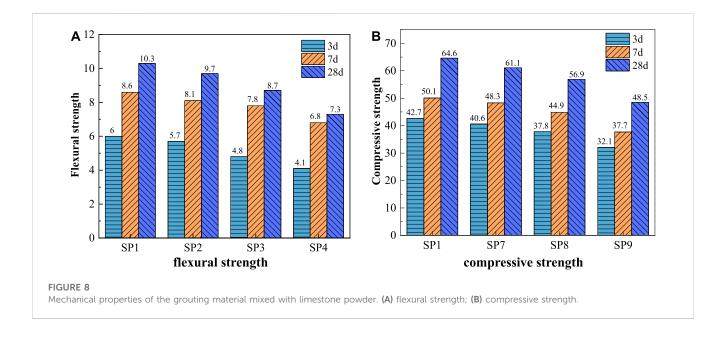
29.13%, respectively; It can be seen that with the increase of the amount of limestone powder, the flexural strength of the grouting material gradually decreases. However, when the amount of limestone powder is less (5 wt%), the flexural strength of the grouting material is only reduced by about 5%.
