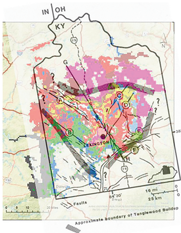
Fig. 6. Superposition of the Lexington area structure map from Ettensohn et al. (2004) on a 3-D raster-file map (Fig. 5), showing patterns that correlate with known structures.
