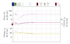
FIGURE 14: Incremental conductance experimental results.
