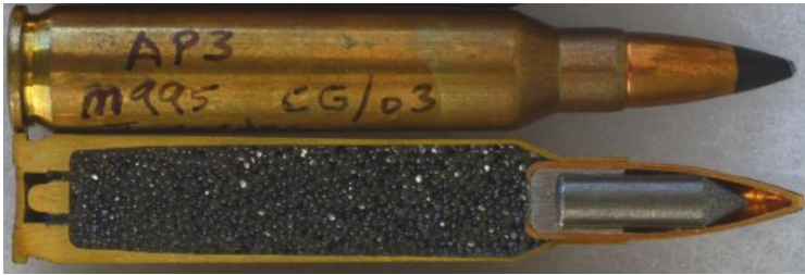
Fig. 2. 5.56 × 45 mm M995 AP3 cartridge, Below - cross section of the round ( www.forum.cartridgecollectors.org )
