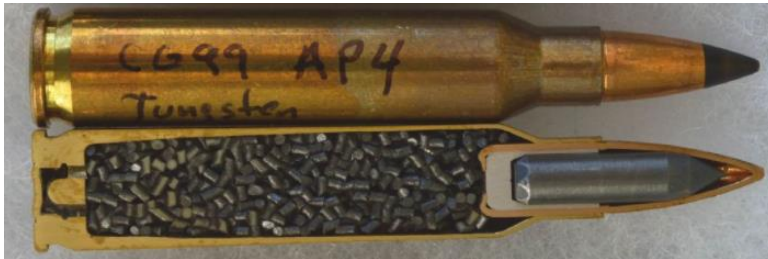
Fig. 3. 5.56 × 45 mm AP45 cartridge, Below – cross section of the round ( www.forum.cartridgecollectors.org )
