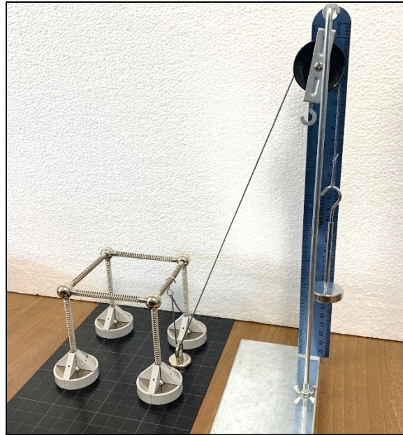
Figure 2 - Mola model and test setup for portal frames exercise (Activity A)
