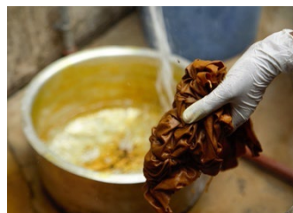
Dyeing batik using natural dye extracted from turmeric root
