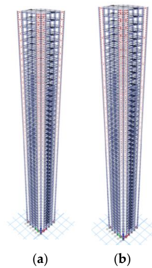
Figure 5. (a) G + 50 shear wall with opening 3D Model Case-2; (b) G + 50 shear wall with opening 3D Model Case-3.
