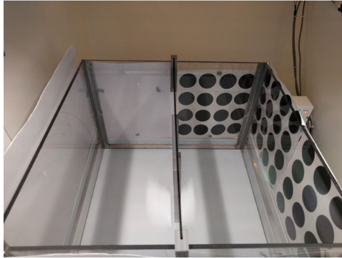
Figure 2: CPP apparatus. Modified open field box (43.2 x 43.2 cm) divided into two compartments (21.6 x 43.2 cm) with white walls on the left side and white walls with black spots on the right.
