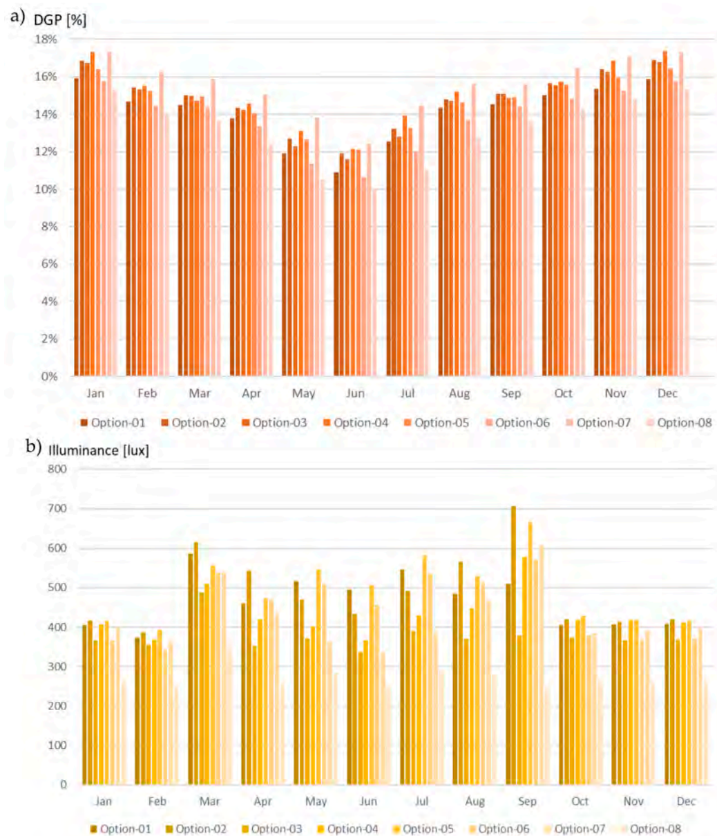
Figure 13. Monthly analysis of different options' effect on average DGP (a) and mean UDI-autonomous range (b).
