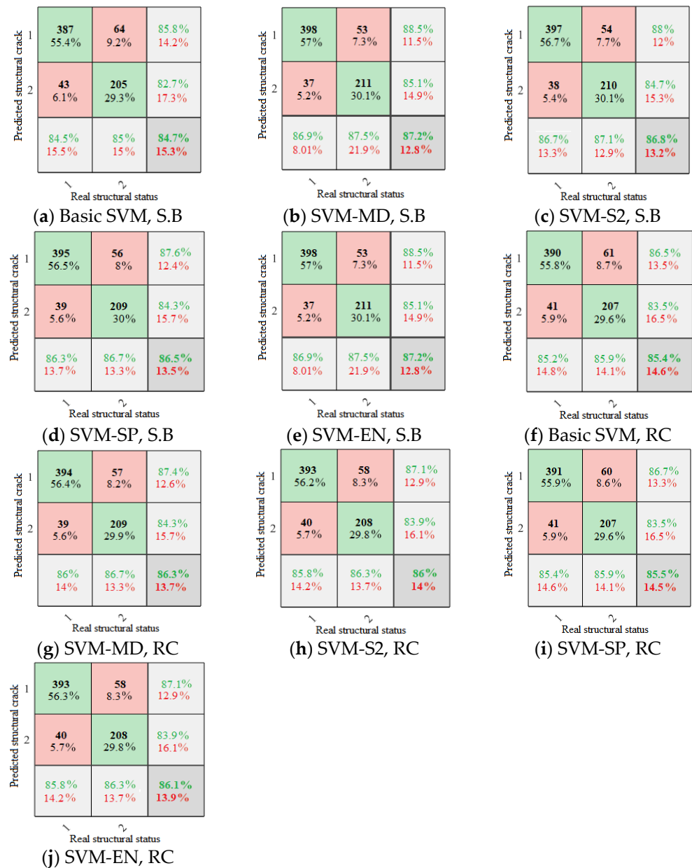
Figure 8. Confusion matrix of enhanced SVM models for S.B and RC beams. The rows correspond to the true class, while the columns correspond to the predicted class. Diagonal and off-diagonal cells correspond to correctly and incorrectly classified observations, respectively.
