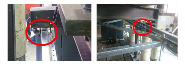
Figure 4-8: Crippling of load points: (A) Typical crippling at flanges; (B) Specific crippling reinforcement.
