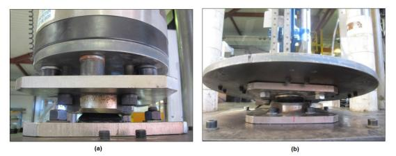
Figure 3-8: (a) Ball bearing; (b) cap plate.
