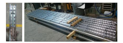
Figure 3-5: Reinforcement along the upright length by bolts and spacers.
