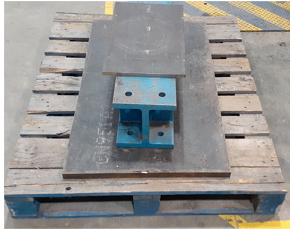
Figure 3. Artificial mass, placed on the test specimen.
