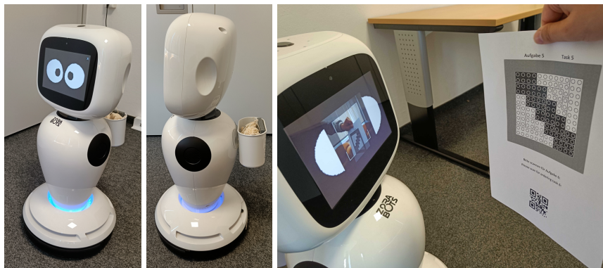
Figure 4. Service robot James with eye animation (left) and the attached backpack (centre). By scanning QR codes, participants could order new material (right).
