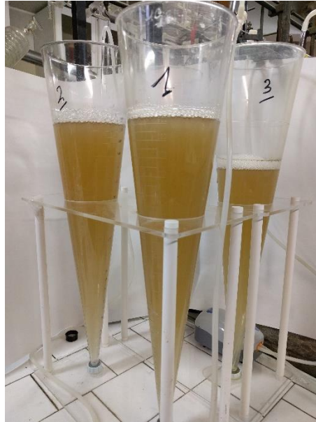
Figure 4.3. Experimental setup of the struvite precipitation process.
