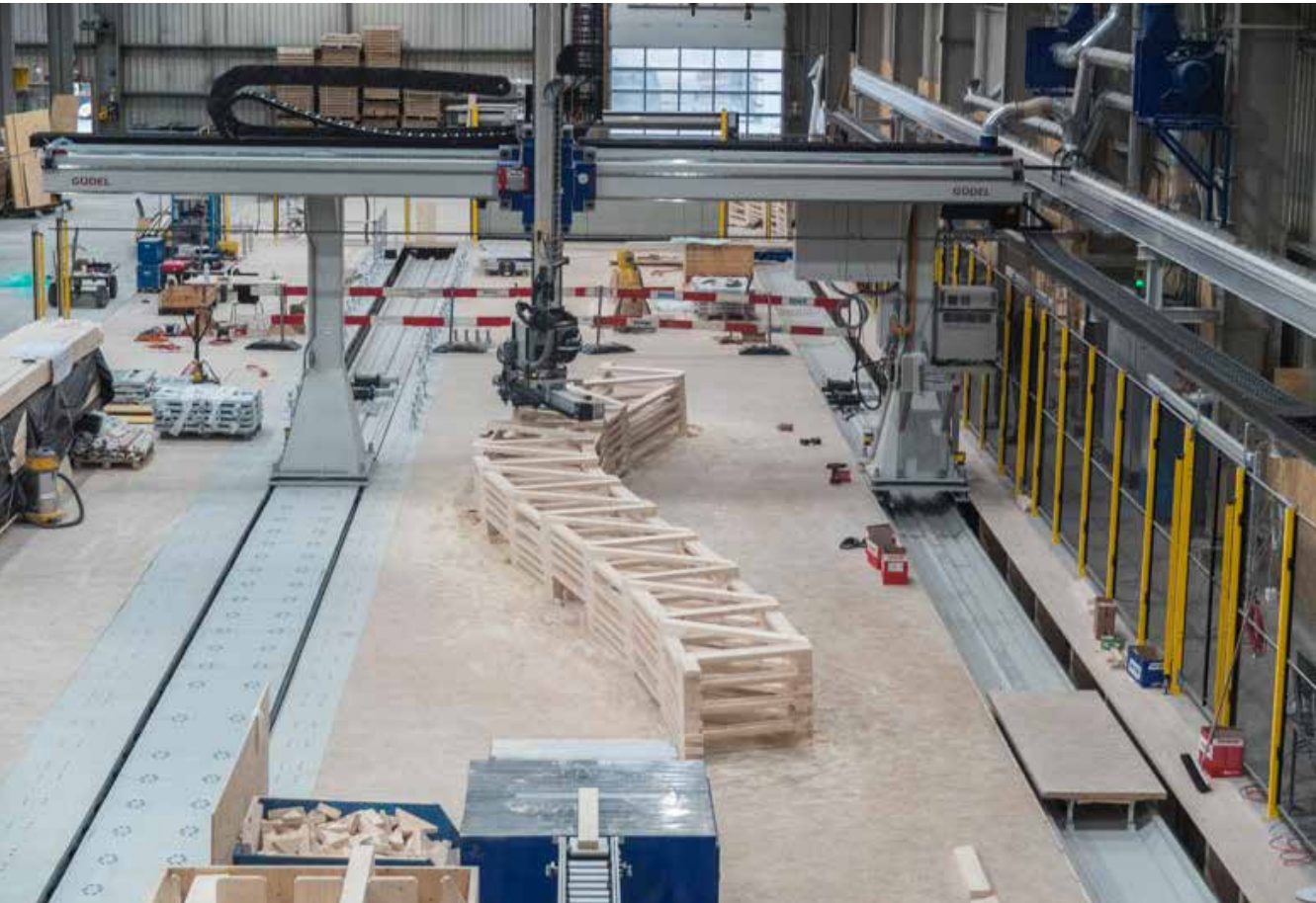
Fig. 5.14 Set-up of the laboratory with the 6 axis gantry robot working on one of the beams.
