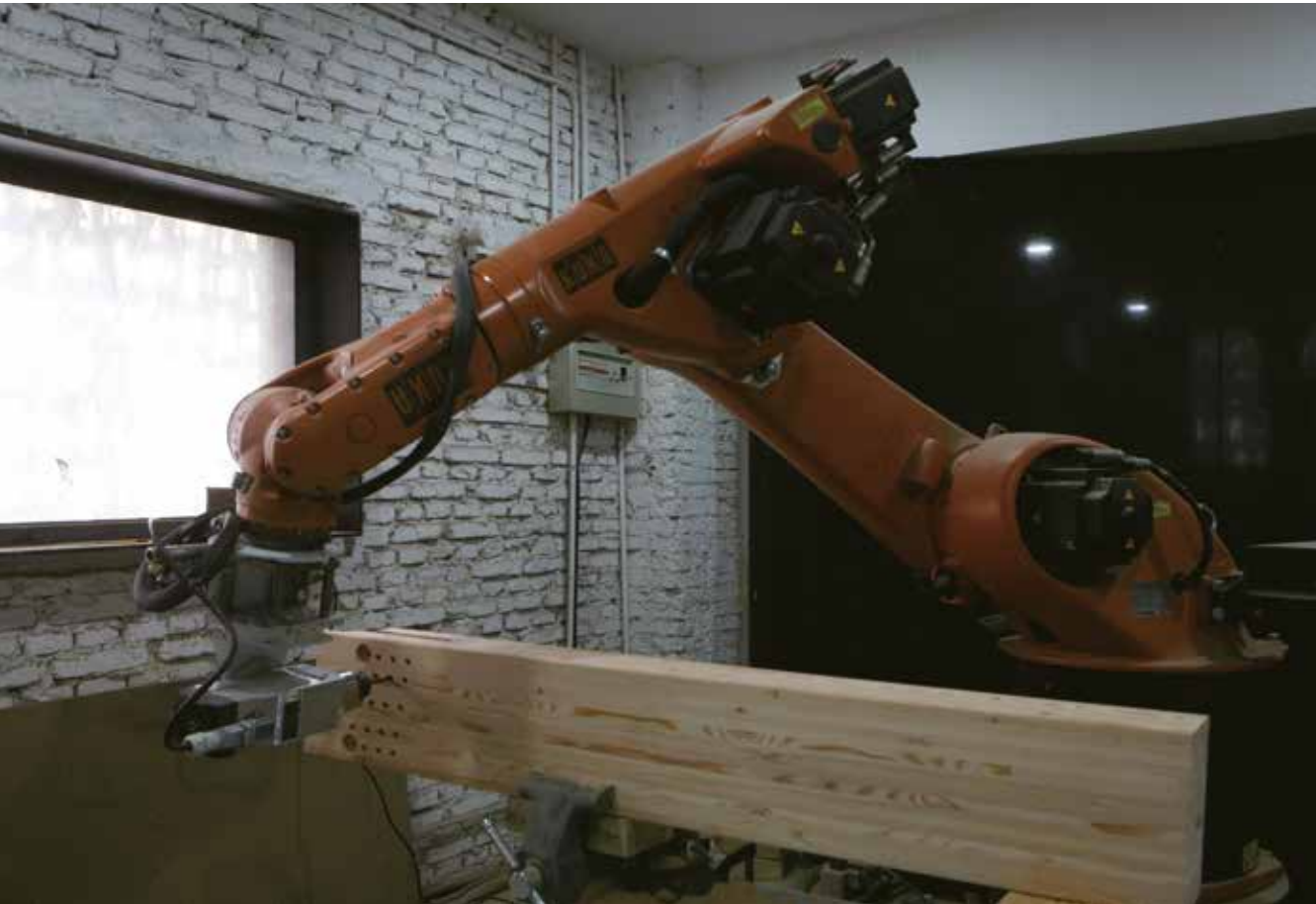
Fig. 5.27 Robotic drilling of a beam for the gridshell pavilion of Suzhou Horticultural Expo
