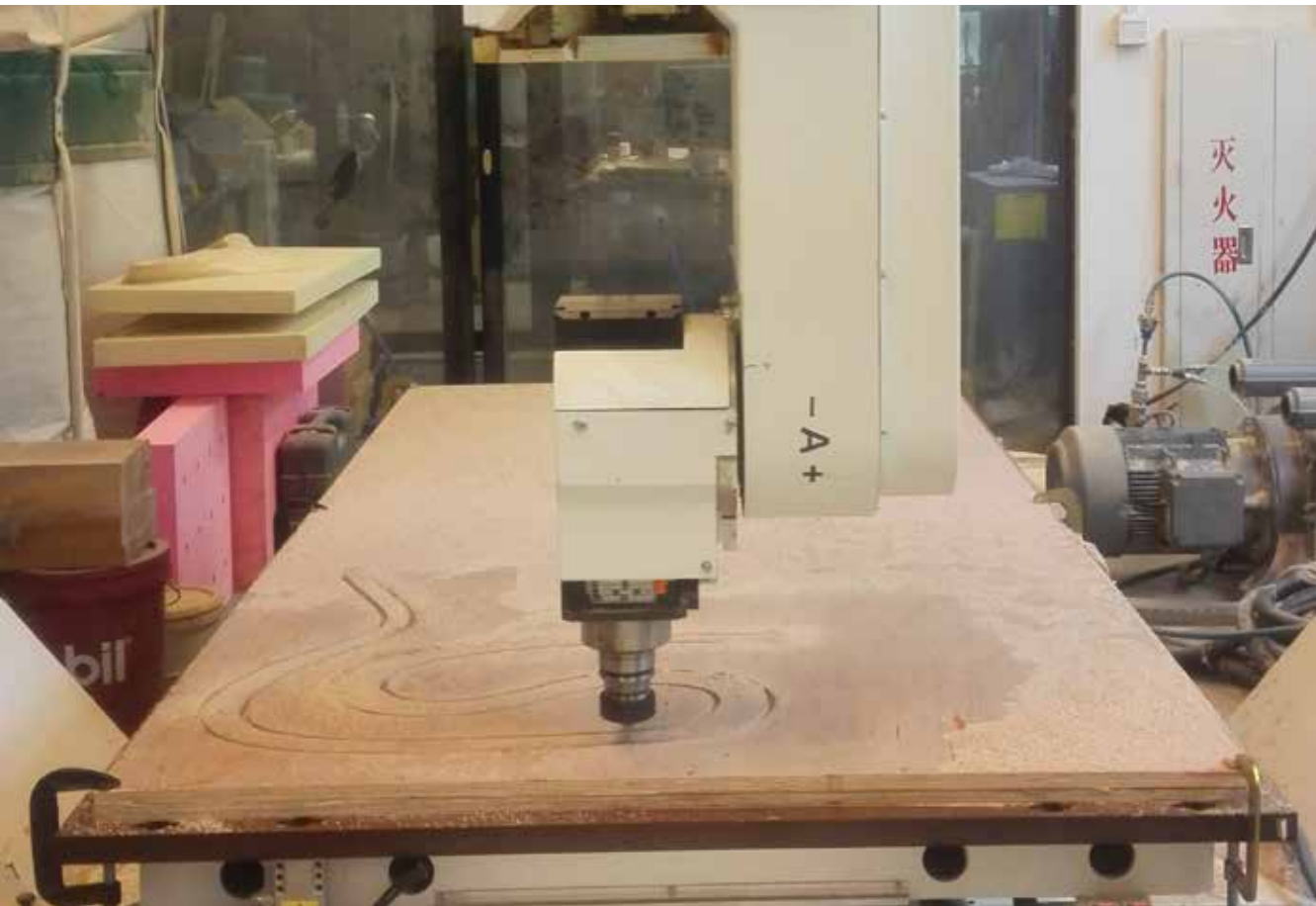
Fig. 6.8 Fabrication of the section on 18mm plywood panels with a 5 axis CNC machine of the DDRC (Digital Design Reserch Center) of Tongji University Shanghai
