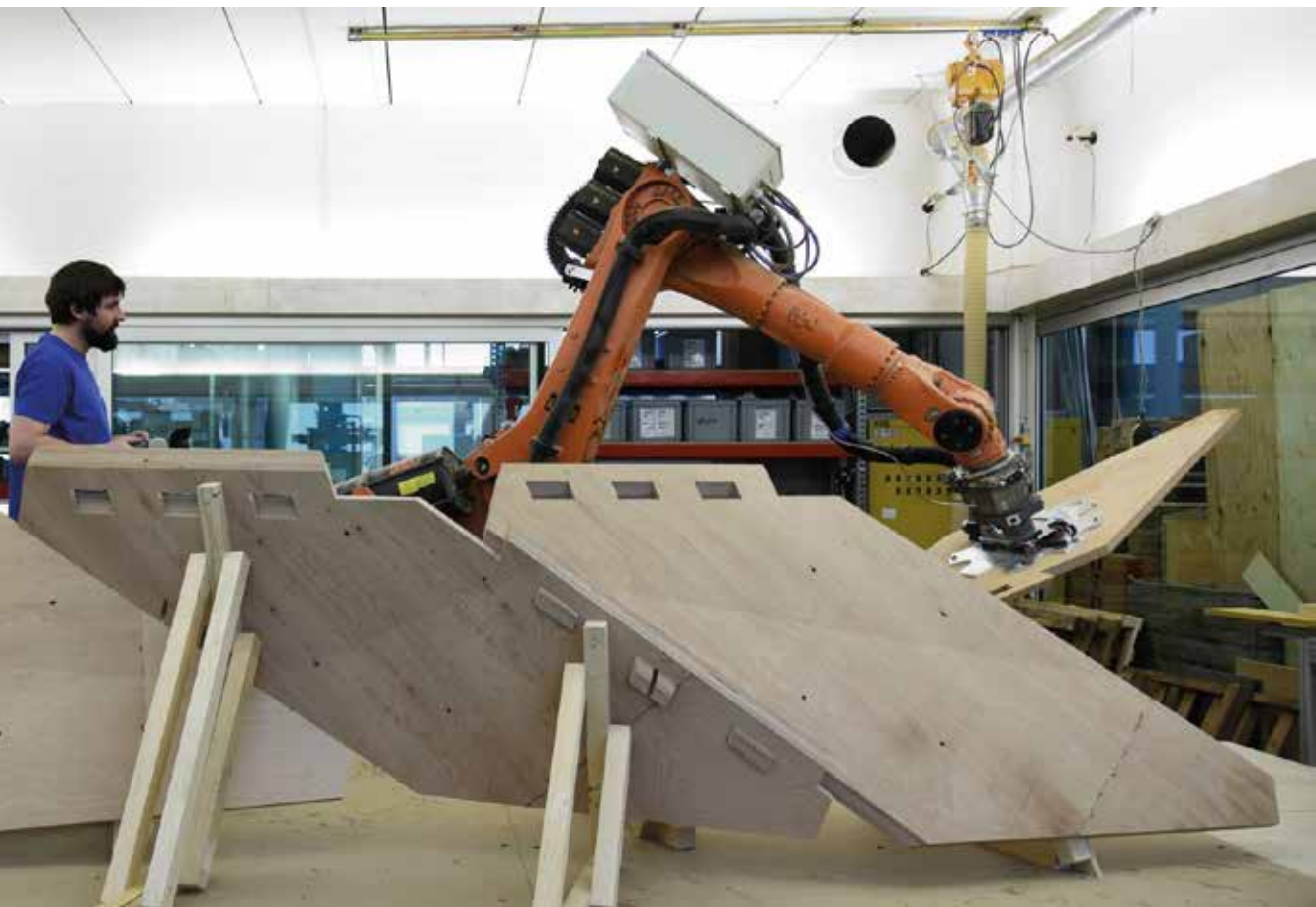
Fig. 5.22 Robotic assembly of timber plates with integral mechanical attachment of through-tenon joints, developed by IBOIS laboratory at EPF Lausanne and ETH Zurich
