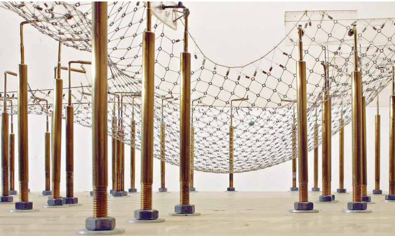
Fig. 4.5 Hanging chain models are often used as form-finding methods. The structure of many projects by Frei Otto are based on this approach and they find their scientific reference in the Hooke’s Law.
