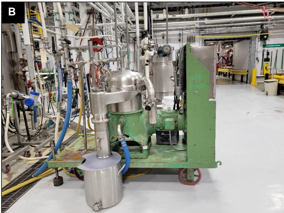
Figure C3 Centrifuges used in the scaling up trials. A) Decanter centrifuge (EC3) and B) disk stack centrifuge (DC2)
