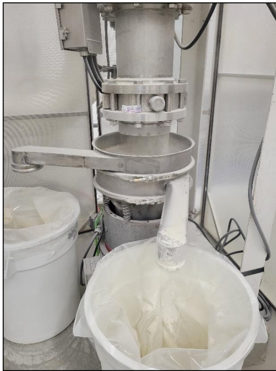
Figure C6 Spray drier outlet showing dried product collection set up (inside the tent shown in Figure 5). A SWECO® Vibro-Energy™ Separator was used to screen clumped particles and any larger foreign material
