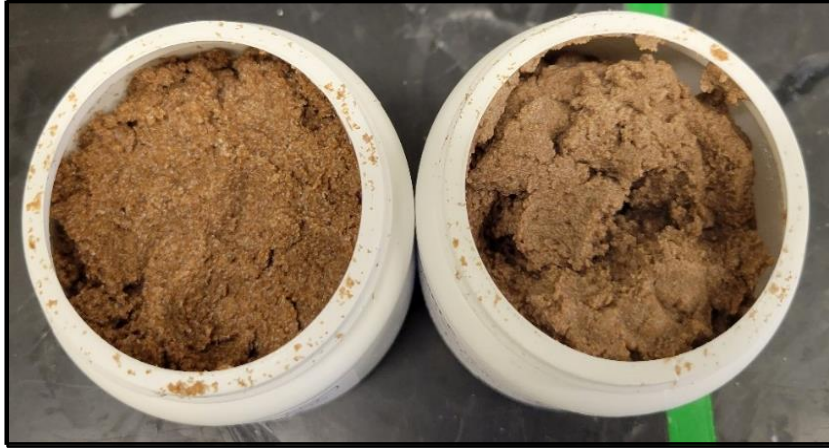
Figure 6.4 The fiber fraction resulting from #60 mesh overs (left) and #165 mesh overs (right)
