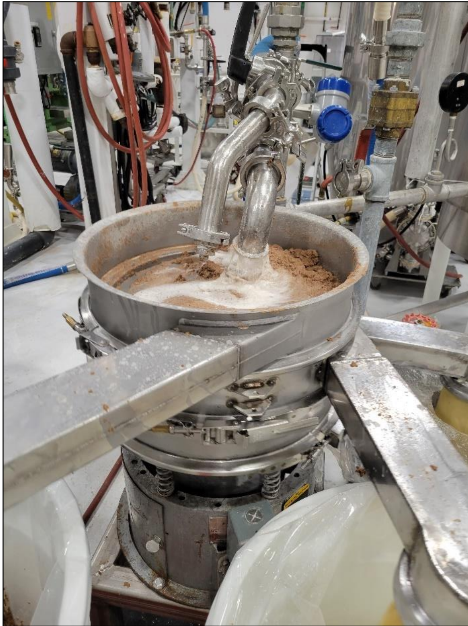
Figure C4 SWECO® Vibro-Energy™ Separator (VS4) set up for screening fiber in the white-flour slurry.
