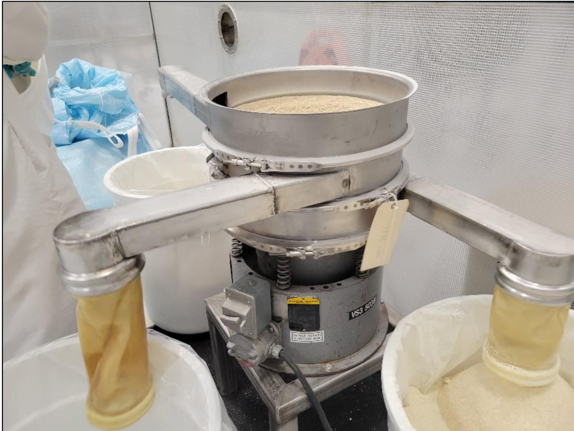
Figure C1 SWECO® Vibro-Energy™ Separator (VS3) set up for canary seed white flour preparation with #24 mesh on the top and #32 mesh on the bottom
