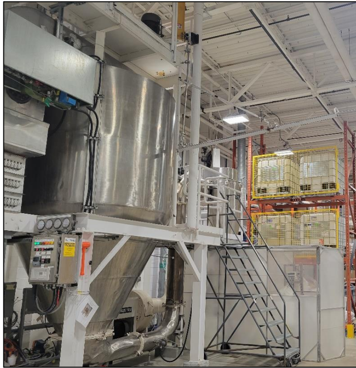
Figure C5 Komline-Sanderson No. D-19 Spray drier (SD1) with the tent covering spray dried powder collection area
