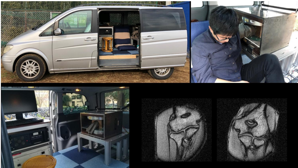
Figure 2.5: Some images of the Baseball Elbow MRI system, the minivan it was installed in and the elbow images it is able to provide. Image and caption reproduced from article [16] with permission (license number: 5357410297482) from publisher: 'Elsevier'
