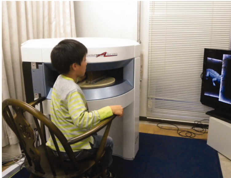
Figure 2.7: Overview of an open, compact MRI scanner used on a volunteer patient. Image and caption reproduced from article [20] with permission (license number: 5357420828479) from publisher: ‘John Wiley and Sons’.
