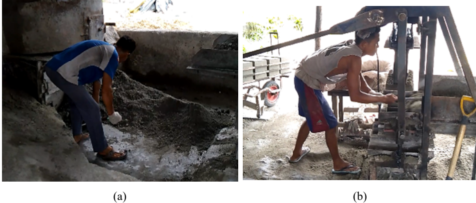
Figure 1 (a) Workers groups sand in bent position (b) Workers filling moulds paving block in bent position (see online version for colours)
