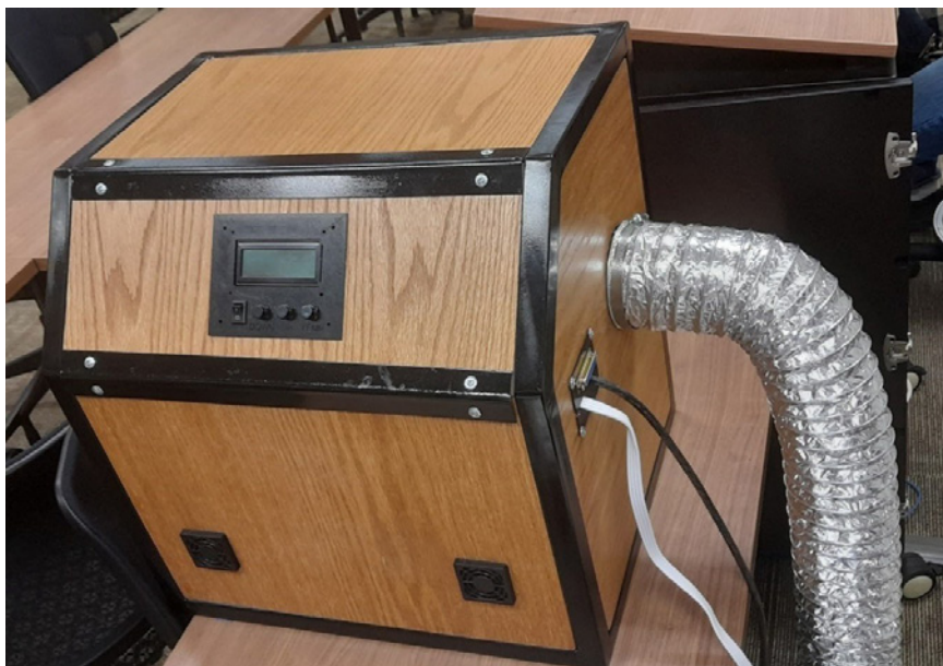
Fig. 16. Final portable air-conditioning unit showing the LCD screen and the duct that connects to the blanket [5]
