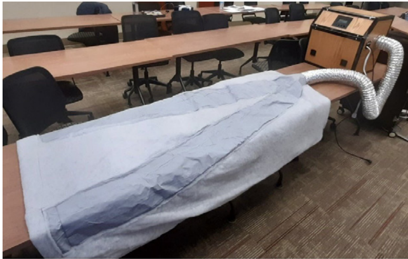
Fig. 15. Final product with enclosure over main unit and showing the thermally controlled blanket [5]
