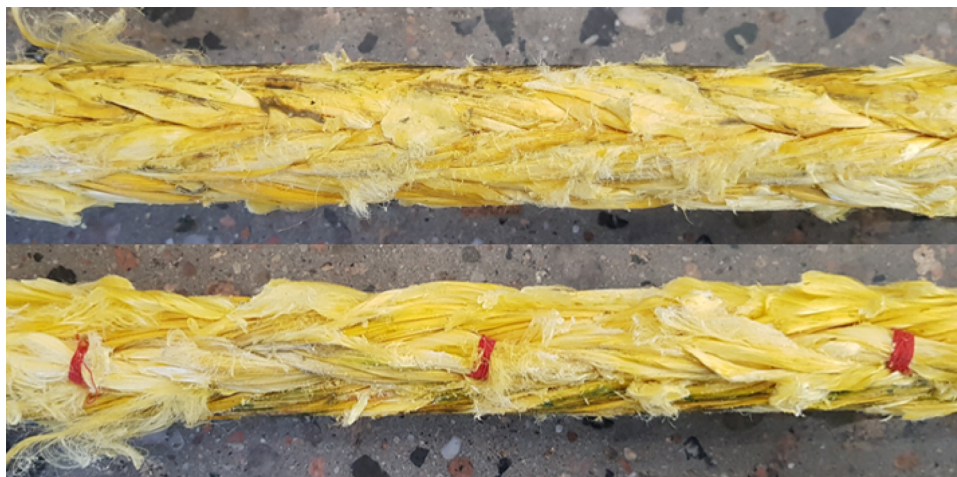
Fig. 8. Compression damage (top) and extruded loops (bottom).
