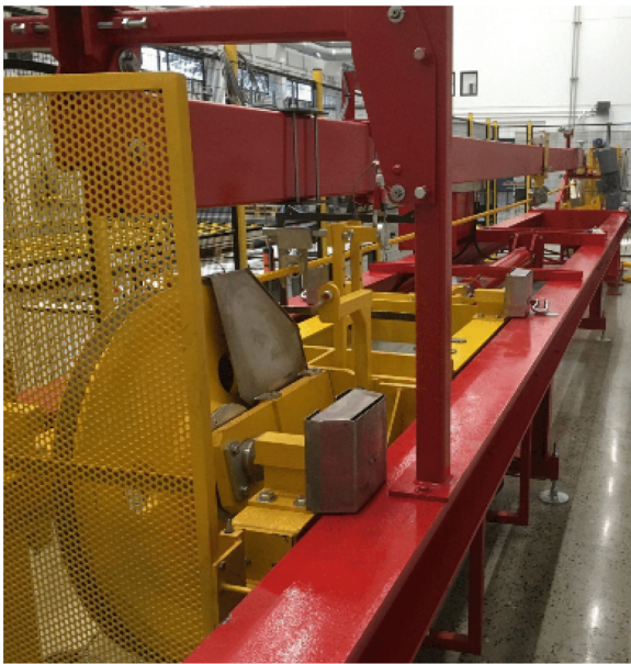
Fig. 1. CBOS test machine as located the MIL, Norway. View is from just behind the test sheave with the driving sheave visible at the far end of the test frame.
