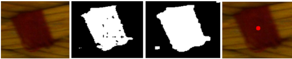
Fig. 4. Different stages and effects of morphological operations applied to the image to detect a specific colour for length measurements: (a) original image, (b) binary image created, (c) dilation operation applied and (d) final processed image with centre point of marker visible after contouring operation.
