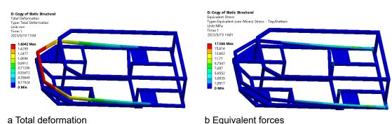
Figure 4. Static properties under torsional conditions
