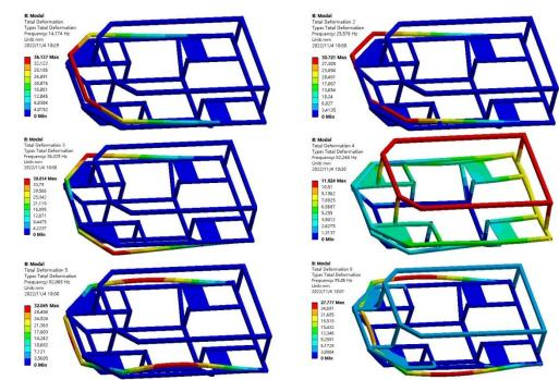
Figure3Displacement modes of steps 1-6
