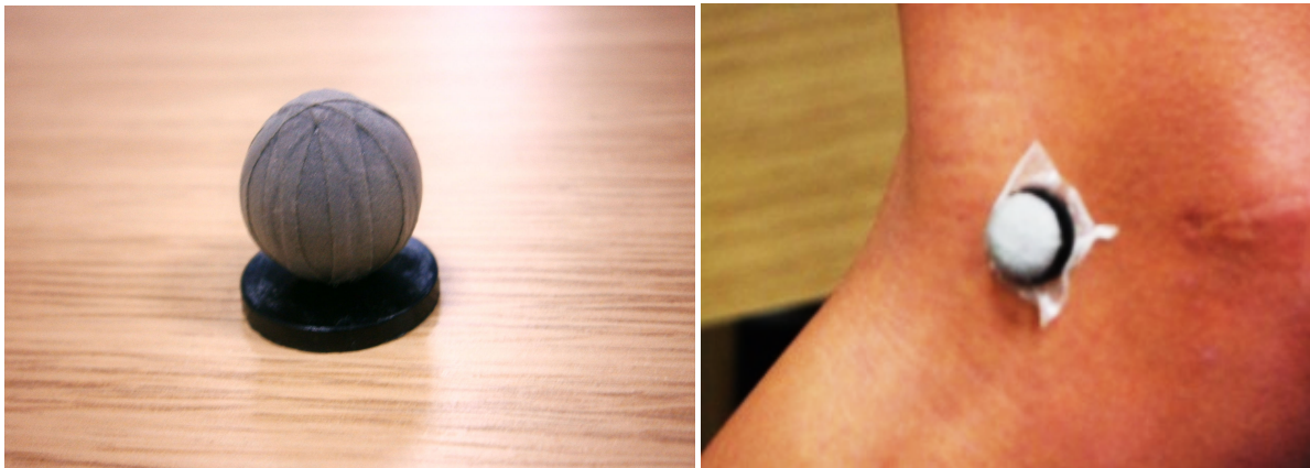
Figure 18. Reflective marker used during Gait Analysis. 20 Reflective markers are used on each participant.
