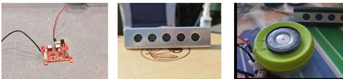
Figure 4: Images left to right – Amplifier evaluation board, broadside microphone array and mini-
