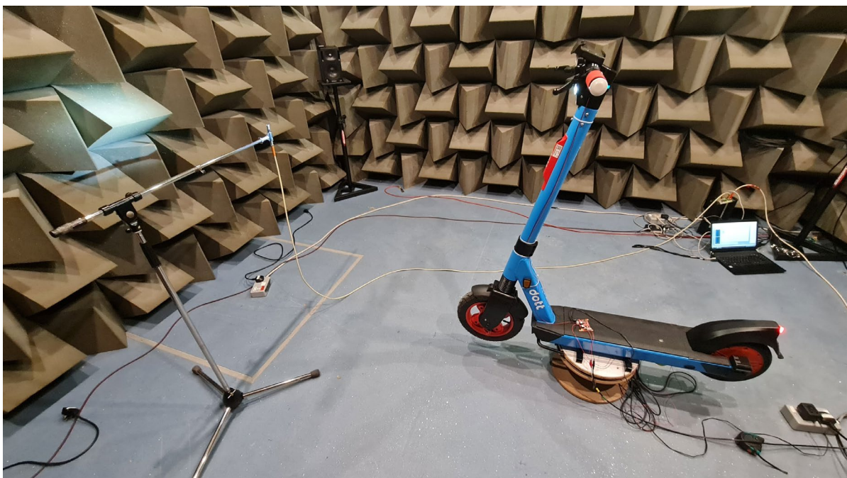
Figure 5: Dott scooter instrumented with forward firing microphone array and mini-sub for testing of sound level and directivity in the semi-anechoic chamber. The scooter is mounted on a rotating platform to allow small, measured rotations relative to a fixed microphone position.
