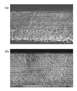
FIG. 2. SEM images of cleaved cross sections of the AB and BA structures. The interface in the AB structure (a) is clearly defined whereas that for the BA structure (b) shows evidence of sagging within the B layer.
