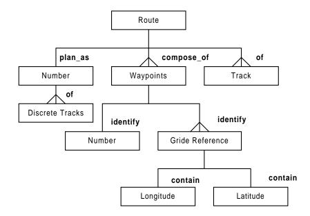
Figure G.1: The ER Diagram of route planing system
