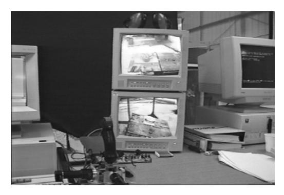
Figure 6.2: View of the operator workstation, showing the camera monitors and the haptic joystick
