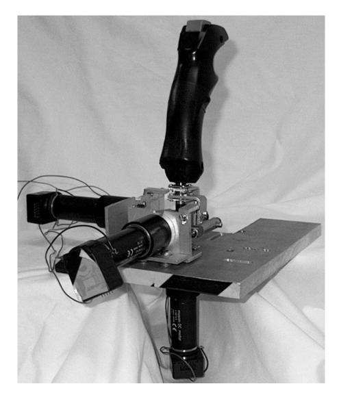
Figure 4.17: The complete three degrees of freedom haptic device
