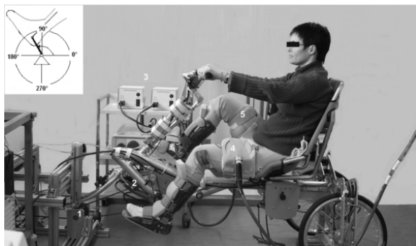
Fig 1. Principle of FMS propelled cycling: complete paraplegic subject
