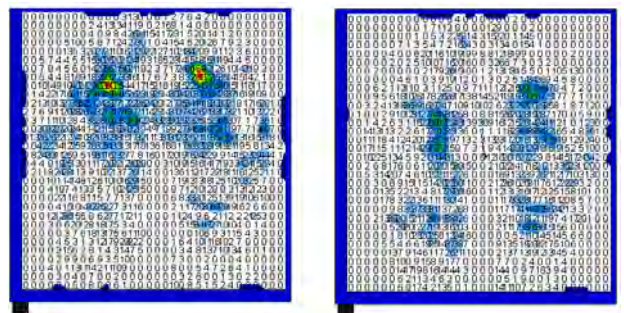
Figure 2: Interface pressure of sitting SCI individuals without and with ES of the hamstring and gluteal muscles.
